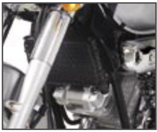
Air/Oil cooling system
