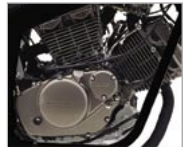
75° V-Twin DOHC engine (125/250cc)
