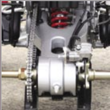
Large rear disc brake and chain guard
