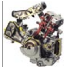
DOHC 90° V-Twin 650cc engine
